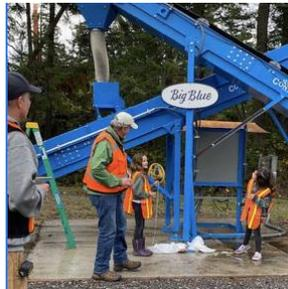
*Orcas Recycling Service's "Big Blue" crushes glass — bottles, jugs, jars, window glass, mirrors — into various sizes. It stays on the island for use by contractors and construction companies, eliminating the need to transfer a commodity with little to no value off the island.*
